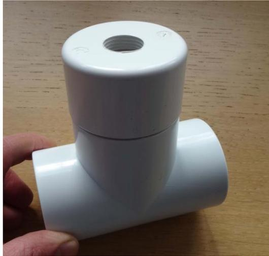
15. Drill a hole in a pool pipe fitting eg elbow or straight connector or the end-cap to suit a 3/8" BSP tap
