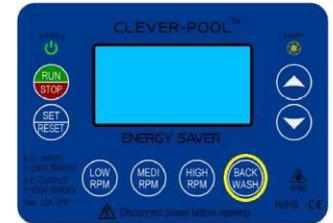
Press the RUN/STOP button to put it into on mode, this will start the pump.
