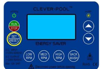
Press the SET/RESET button to step to SPEED setting. The display will now show the flashing four digits for speed, which is the speed for AUTO MODE 1. Press the up or down button to change motor speed. Alternatively press one of the pre-set speed buttons LOW RPM, MEDI RPM, HIGH RPM.
